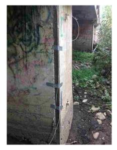
Figure 134. Attached Accelerometers on the Pier Side
