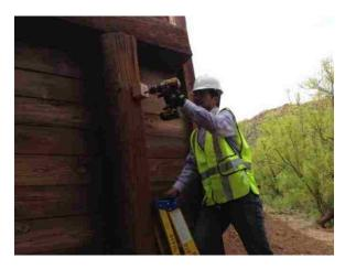
Figure A13. Attaching the Striking Block on the Test Pile
