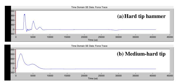
Figure 72. Impulse Signals of Striking on an Aluminum Block
