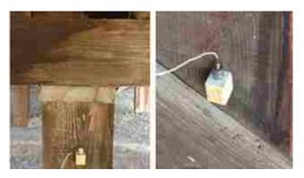
Figure 26. Accelerometers Mounted on a Pile by Wooden Blocks.
