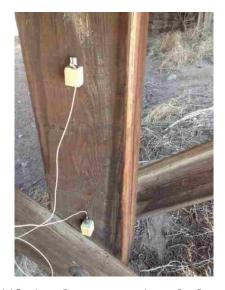
Figure 118. Accelerometers Attached onto a Pile
