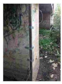
Figure A19. Two Accelerometers Mounted on the Side of the Substructure
