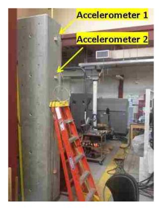
Figure 45. An SE Setup on the Reinforced Concrete Wall
